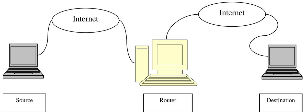
Considering the above figure, Source and Destination are two hosts separated by either one or more networks. The Router is a host on one of the networks between Source and Destination also Router forwards the packets from the Source to Destination and vice-versa. My software which is loaded at the Router adds a new capability to it. This capability is to drop the first n packets of the flow from Source to Destination which contains a particular string in the TCP Data.
